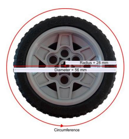
How far will the robot travel in 2 rotations? Answer: 2 times the circumference of the wheel. The wheel is the tire and the rim.
